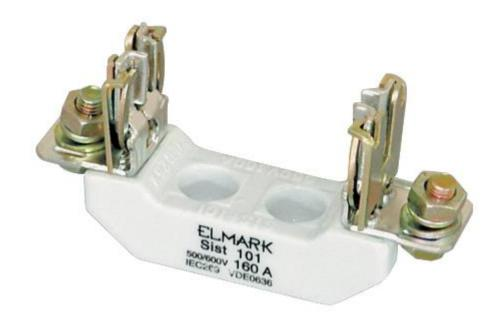
The series bases for high power safety device is manufactured of permitivity alloy with mounted contact jaws of electrolytic copper supplied with special springs for contact compression and easy fuse links taking out. All current leading parts are connected to inlet outlet terminals with bolts; the terminals also end with bolts, to which the power supply conductors are connected. The bases are offered in five type sizes corresponding to the five types of fuse links.
